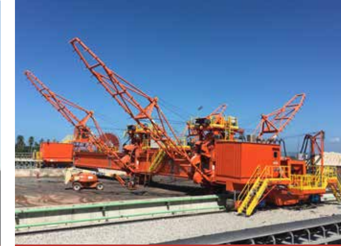
Köprü Tipi Kovalı Toplayıcı Bridge Type Bucket Wheel Reclaimer
