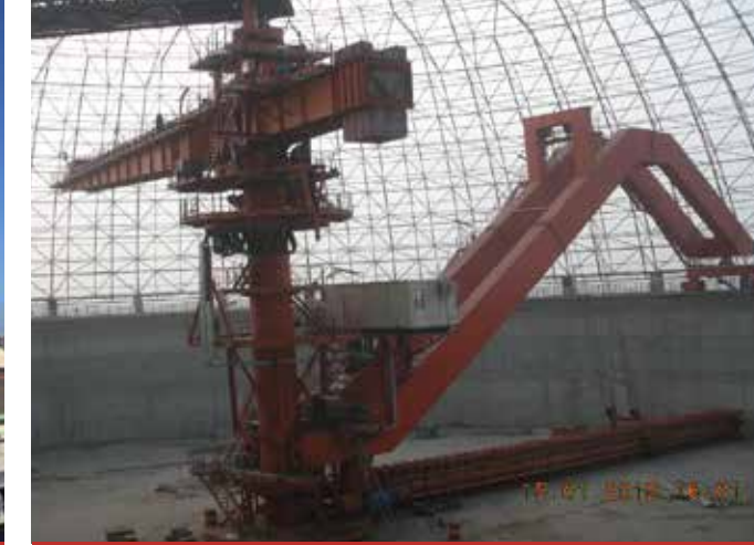
Dairesel Tip İstifleyici Toplayıcı (Yan Tip) Circular Type Stacker And Reclaimer (Side Type)
